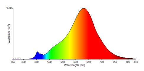
Testing was performed in accordance with LM-79-08.
